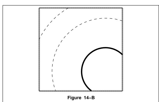
A Graphical representation of the occulting disk edge (innermost arc with the solid dark line) and the inner and outer edges of the Lyot ring (slightly enhanced optical brightness), which are indicated by the dashed arc lines.
